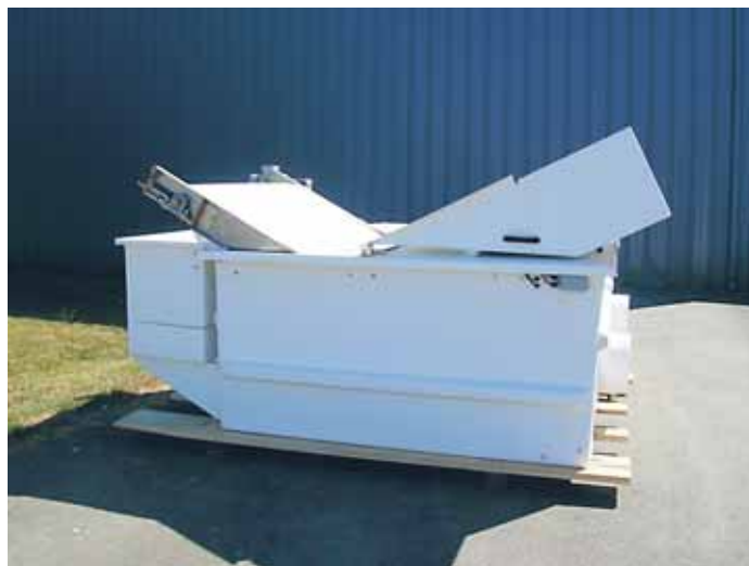
Moving screen fish exclusion system
