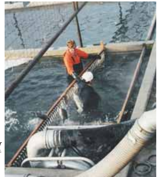
Submersible impeller pump. Note the barrier used for crowding the fish into the pump.
