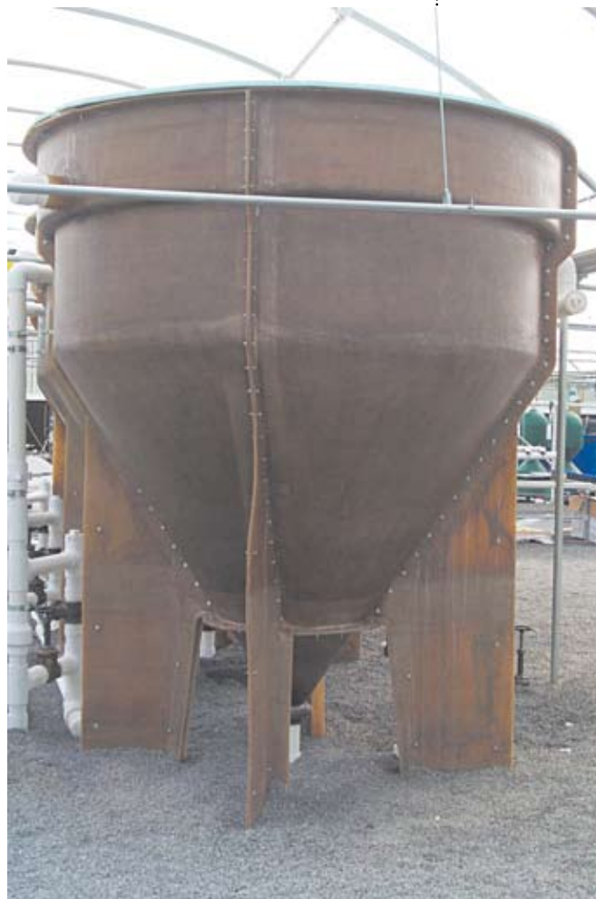
Settling basin. Concentrated slurry is drawn off at the bottom. (Photo courtesy The Freshwater Institute)
