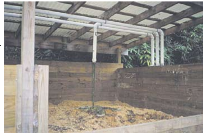
Composting solid fish farm wastes after de-watering. The pipes deliver air for aerating the compost.
