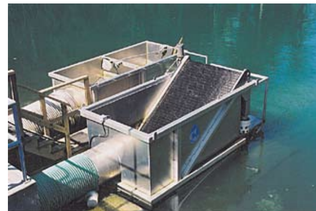
Moving belt filter screens water prior to its entering a settlement pond.
