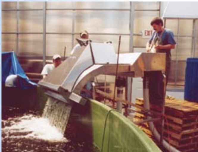
Advanced fish handling equipment, such as counters, graders and fish pumps, may significantly reduce the labour costs of fish handling.
