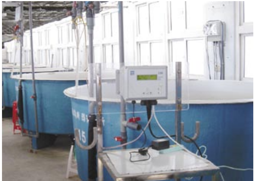
The YSI 5200 Recirculating System Monitor installed in 2004 at a horseshoe crab farm in Taiwan.
