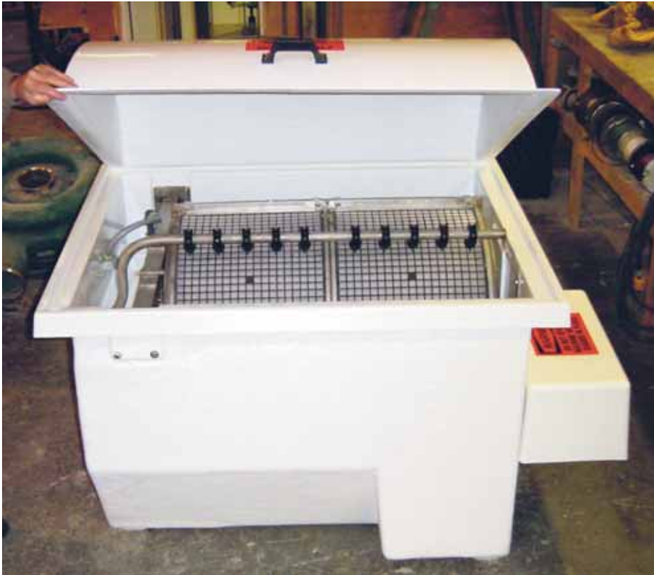
Typical drum filter used for pre-filtration.
