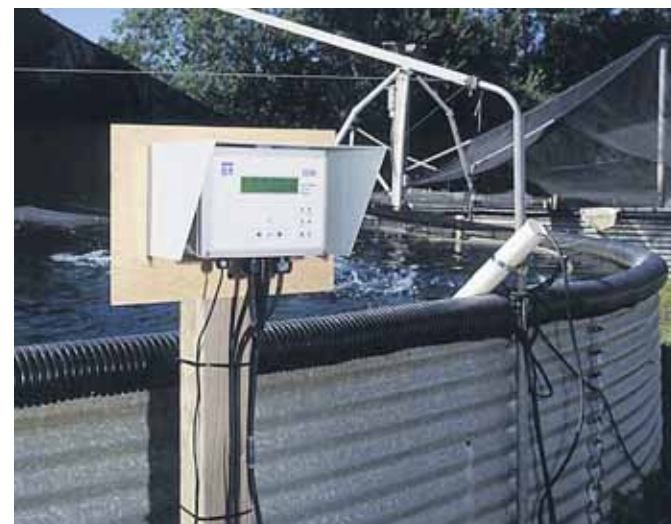
Above: YSI 5200 unit mounted on an outdoor tank.
